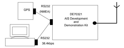
Figure 2 – 'Rx only' Operation using DE70321 and FI-2.x
