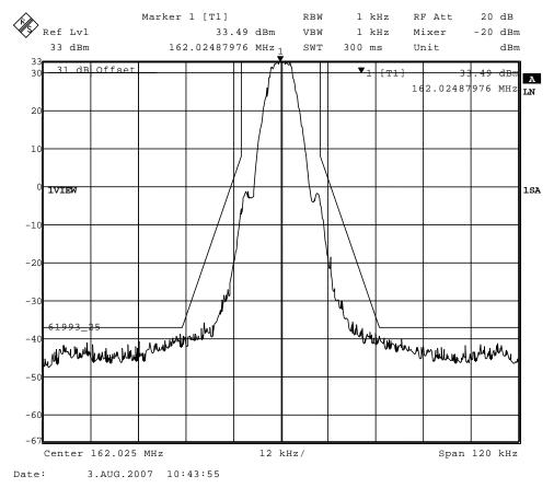
Figure 3 - DE70321 Continuous PRBS Modulated Tx Spectral mask (IEC61993-2, 'Class A') at +33dBm (2W), 162.025MHz
